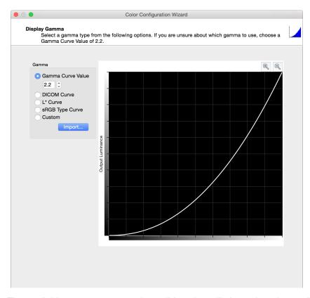
The gamma of a display is the relationship between the video input signal level and the light output (luminance or brightness) displayed on the monitor.
