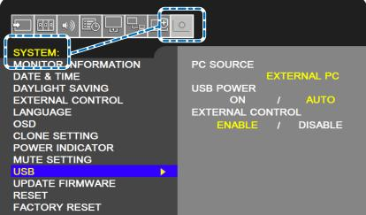
Step 2 - in the OSD menu, enable USB control of the display from the connected PC.
