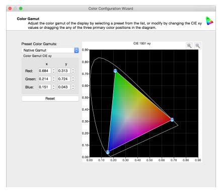
The color gamut is the range of colors that can be displayed by the monitor. The color gamut of a monitor is defined and bounded by the red, green, and blue primaries which together make up all other colors. The SpectraView Engine is capable of manipulating these primary colors in order to display different colorspaces.
