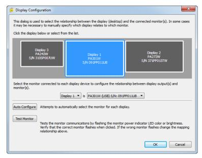
If more than one display is being used, it may be necessary to manually configure the relationship between the display layout on the desktop and the displays that are connected to the system. Correct configuration of this relationship is necessary so that the display adjustments are sent to the correct unit, and that the generated ICC profile is associated with the correct display.
